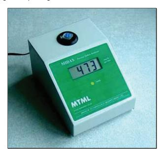
Manor Technology has introduced The MIDAS free standing oil sample based ferromagnetic metal debris analyser, to facilitate ferrous debris analysis. The rapid and simple operation of MIDAS is accompanied by supreme sensitivity. MIDAS' cost effective operation enables routine on-site ferrous debris monitoring, and is also a valuable instrument for precision specialist CM laboratory work.
