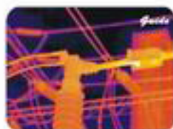
Inspect electricity hot point
